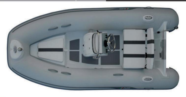
**Overal Length** : 11'6"/3.50m Number of Chambers : 3 Shaft Length : 20" / 50.8cm **Overal Beam Person Capacity** RDC Design Category : C : 5'7"/1.70m : 5
